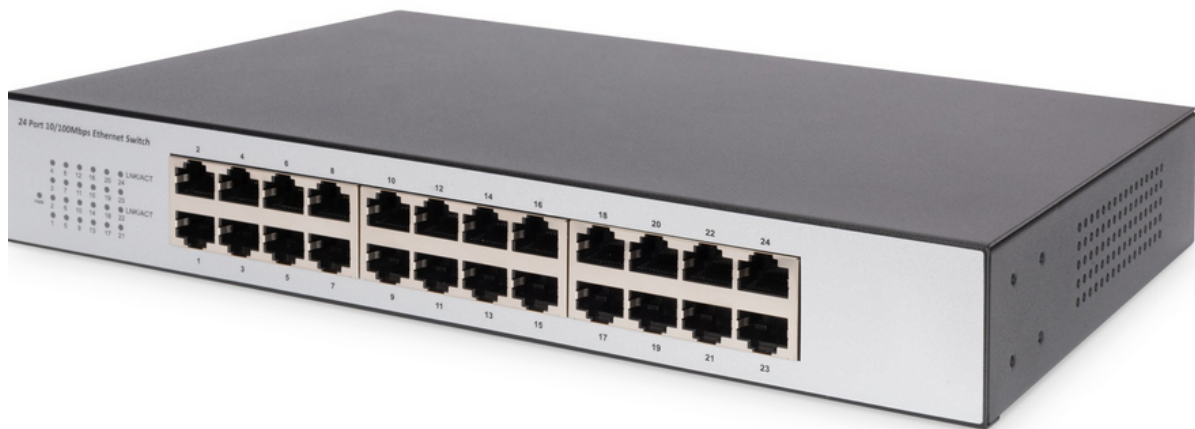
A 24-port switch. Each port connects to a device through a cable
