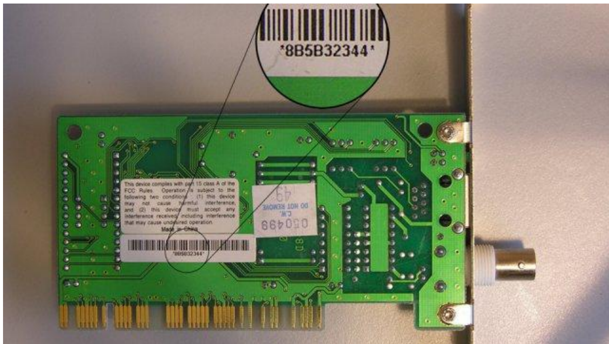
Network interface card showing its specific MAC address
